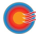
A conventional round pipe creates a 'bullseye' effect whereby the hot water travels down the centre, limiting heat transfer to the surface.
