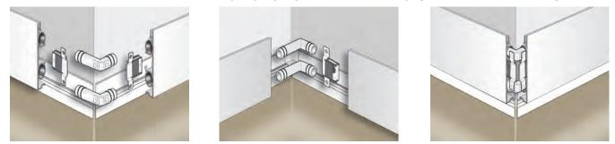
TIP: If any of the mounting rails interfere with the elbows or return manifold, then the mounting rail can be nibbled away using pincers.
