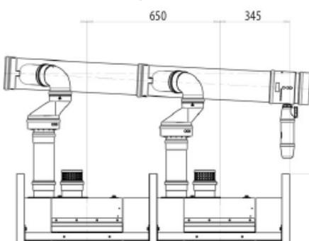
Guidance for boiler/s mounted on and flued through an external wall on a single boiler or cascade boiler installation where each boiler has an individual flue system fitted.
