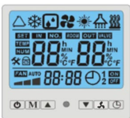
Picture: Display showing all its indication for a moment only when the heat pump receives power supply.
