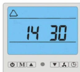
Picture: Parameters check, input water temperature 30°C.
