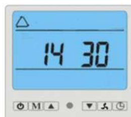
Picture: Parameters check, input water temperature 30°C.
