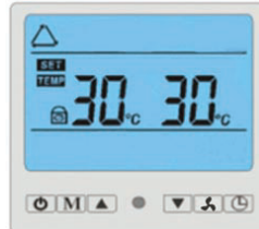
Picture: Child lock activated. A lock icon is showed on the left.
