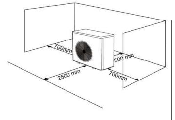
It is advised to install the condensing unit on a **stand 300-500mm above surrounding ground**. Heat pump installed directly on a surrounding ground can by easily immersed into snow and/or into frozen condensation. This can decrease heat pump's efficiency and performance and lead to heat pump malfunction, damage or failure.
