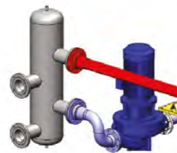
Low loss header Mono header
