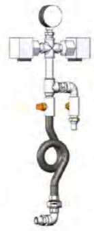
2x max. Water pressure switch + pressure gauge
