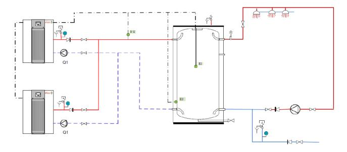
System 3: bypass water heater with buffer tank
