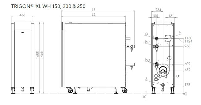
To optimize the position of the boiler in the room it is possible to exchange the position of the electrodes from the right side of the boiler to the left side of the boiler.
