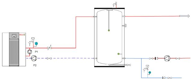
System 5: bypass water heater cascade with 2 buffer tanks
