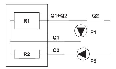
P1 = bypass pump P2 = system pump
